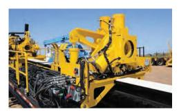
STAY ON SCHEDULE. A floating vise allows the breakout system to clamp the rod fully during breakout, prevent rod wrap and keep your crew on schedule.
