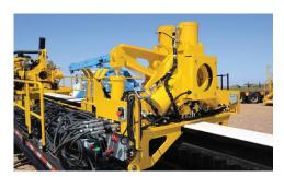
STAY ON SCHEDULE. A floating vise allows the breakout system to clamp the rod fully during breakout, helping to prevent rod wrap and keep your crew on schedule.
